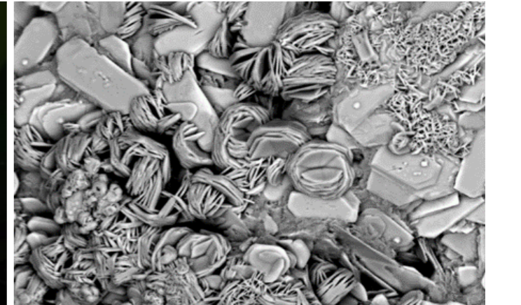
Left: LIBS (Laser-induced breakdown spectroscopy) analyses in a mineral sample. Photo: Andrés Ulloa. Right SEM (Scanning Electron Microscope) image of diverse sulphates
