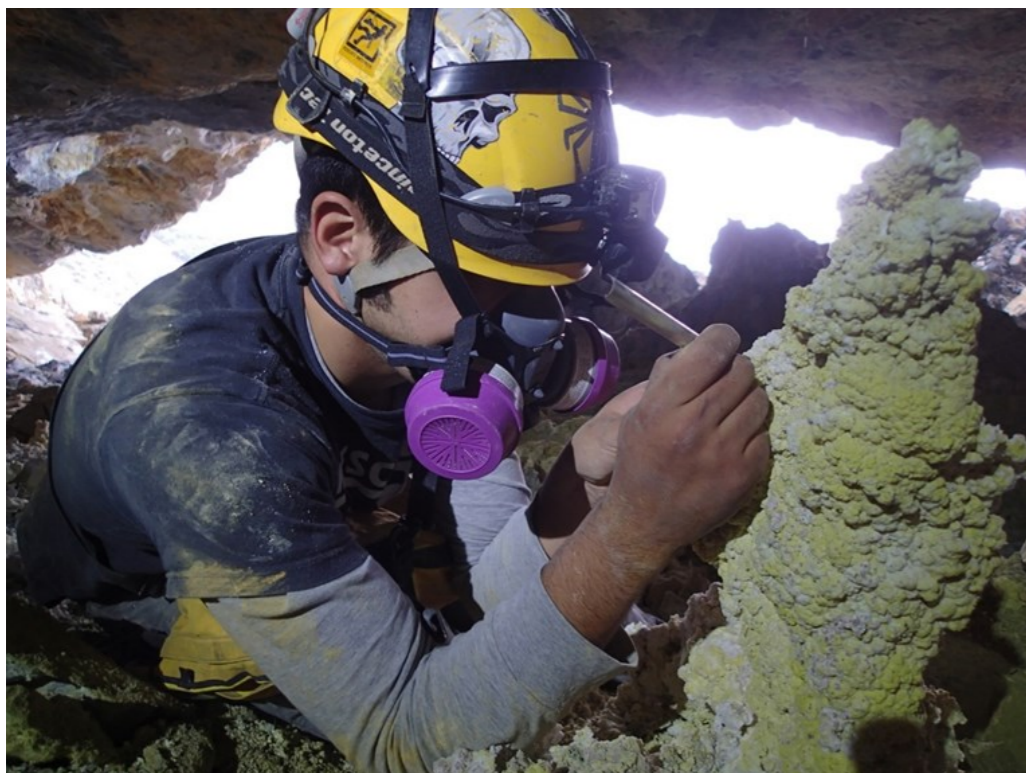
Andrés sampling a geysermite for mineral analyses. Use of mask is necessary in some parts of the cave because of high concentration of volcanic gases. Photo: Scott Trescott
