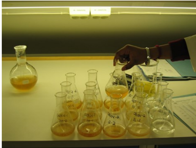
Figure 5. Toxicity testing of whole effluent (here with Skeletonema: marine algae ) gives valuable information of environmental risk
